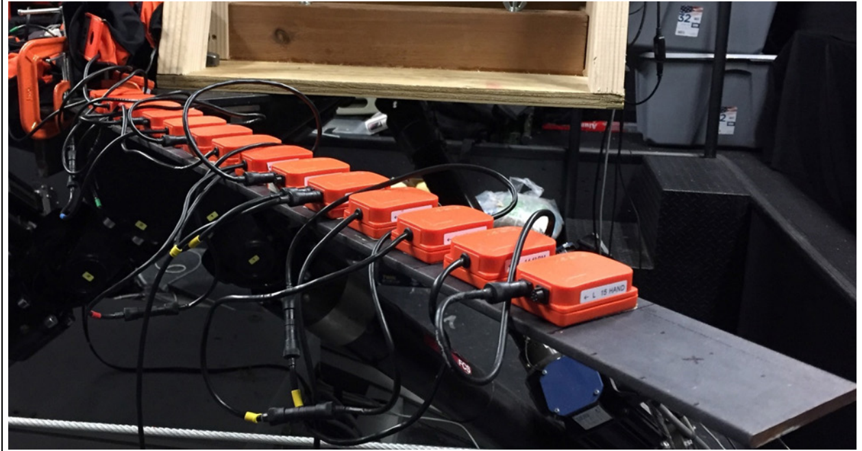
Figure 2-18 Experimental setup of the cantilever beam in the laboratory showing the locations of the fourteen sensors across the cantilever beam.
